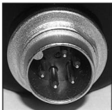
The connector plug is used for communication with a PC / laptop. The interface cable (K-107 / K-104B) can be connected here.
