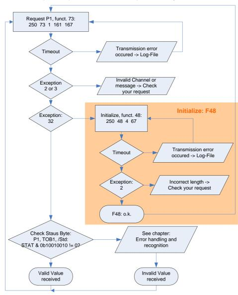
A simple example for reading out a pressure value. Because only one transmitter is connected, the "transparent" address 250 is used. To read out pressure functions 73 and 48 are necessary. When the slave replies with error no. 32 (device just recently started up, power on), then this has to be confirmed with function 48. This is
